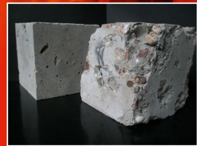
Test specimens after fire testing: specimen with and without fibres.
